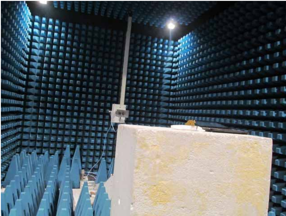
Description: Transmitter Spurious Emissions Test Setup for Above 1GHz
